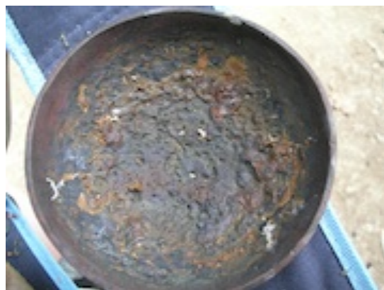
4.4. A hard crust forms on the crucible sides
