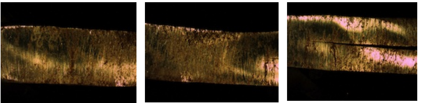
Figure 10. Observations of left, middle, and right sections of Bar II under an optical microscope (Ash 2)
