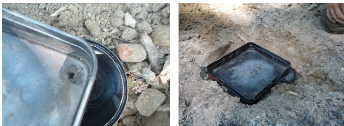
Figure 5. The layout of the containers in order to produce seaweed charcoal and tar
